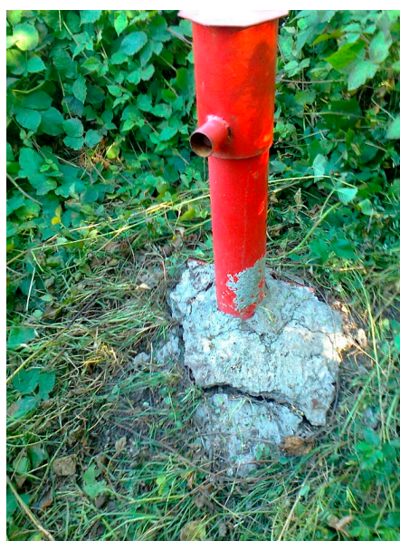
Figure 17. Cracks on concrete at the borehole inclinometer IJ3. The picture shows the ground subsidence of the lower part of the column holding the instrument. Photo: Jan Suchý.
